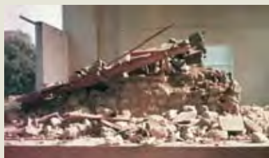
3.3m & n Full-size models of rubble stone low-strength masonry houses, 3.3m with seismic bands, and 3.3n the same construction but without seismic bands. Both were tested on the IIT-Roorkee shock table. Source: Agarwal et al, 2002.
