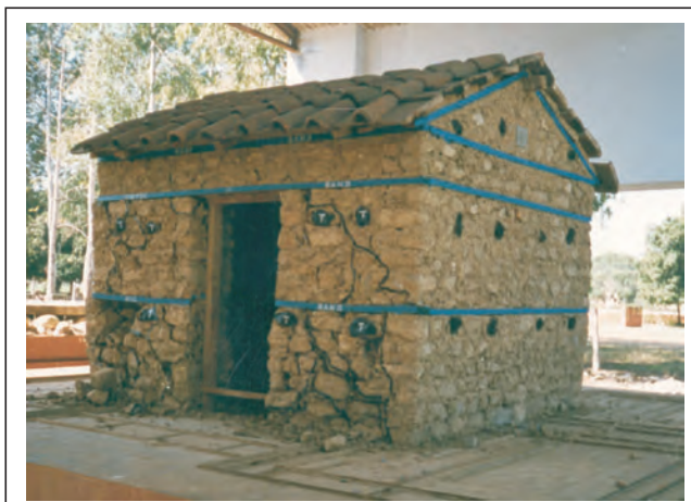
Fig. 8 Positive action of bands reduces damage sharply
